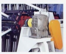
Heavy-duty worm reducer insures controlled indexing, even when rotating an unbalanced load. The caterpillar chain for rotation feeding is heavy-duty and stable.
