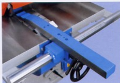
NEW PRECISION GEAR TYPE MICRO-ADJUSTMENT GUIDE FENCE
