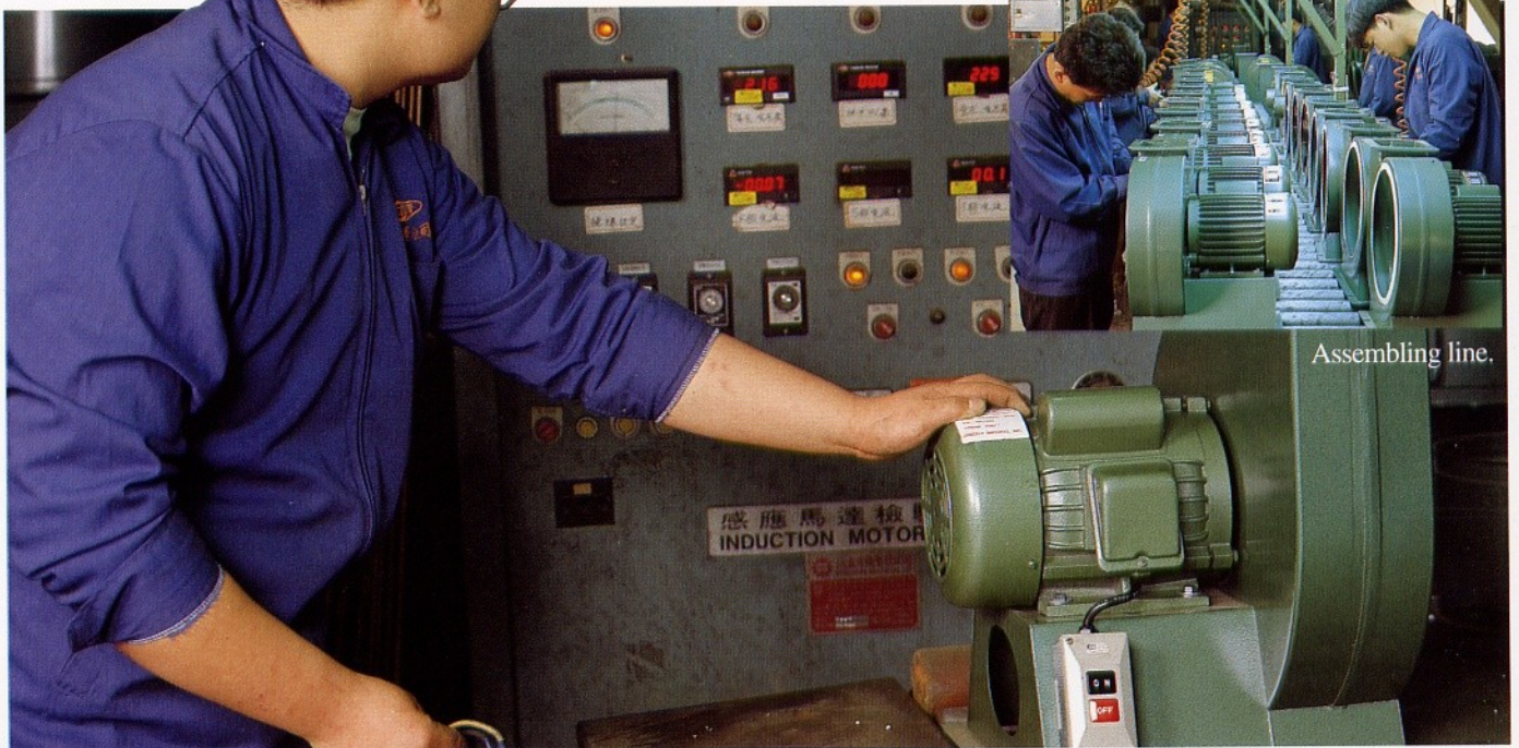
This comprehensive test includes: Wire and connection test, switch wiring motor loading voltage, insulation, and motor running direction.
