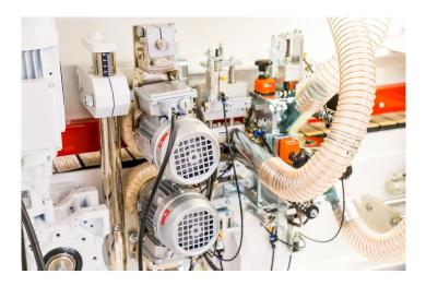
BUFFING UNIT Buffing unit: 2 motors 0.05 kW, 1,500 rpm provide a super-finish for ABS and PVC edge material.
