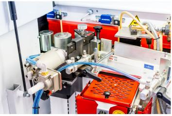
CUT-OFF KNIFE Pneumatically operated cut-off knife from roll material up to 3mm edge thickness
