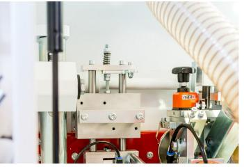
GLUE SCRAPER UNIT removes eventual glue rests with a slight draw cut from the glue joint of the work piece surface
