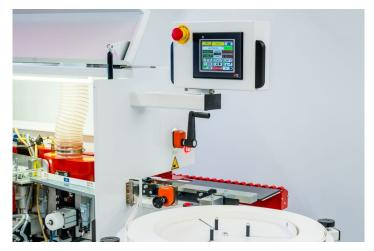
EDGE FEEDING Automatic, timer controlled edge feeding for roller material over turntable  $\mathsf{D}=600\mathsf{mm}$
