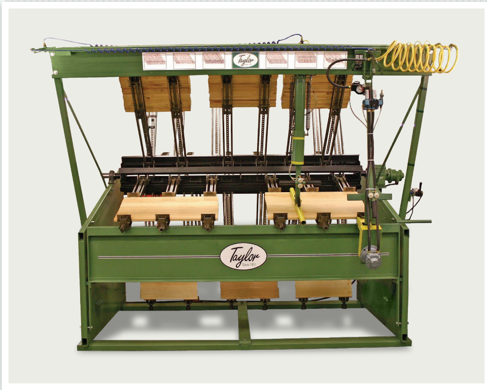
8 1/2' wide Carrier with 3' panels, Swing Style Tightener, Flattener and Motor Drive. (Pneumatic only.)
