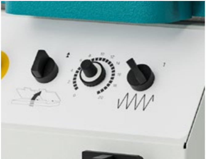
Continuously adjustable feed | T3221
