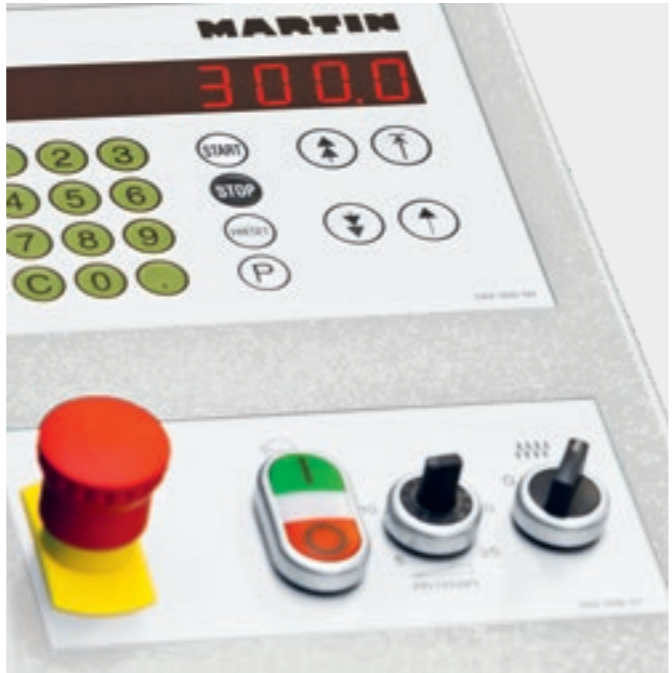
Continuously adjustable feed speed 5 – 25 m/min | T4510
