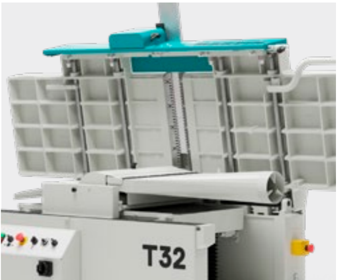
T32 equipped for thickness planing mode
