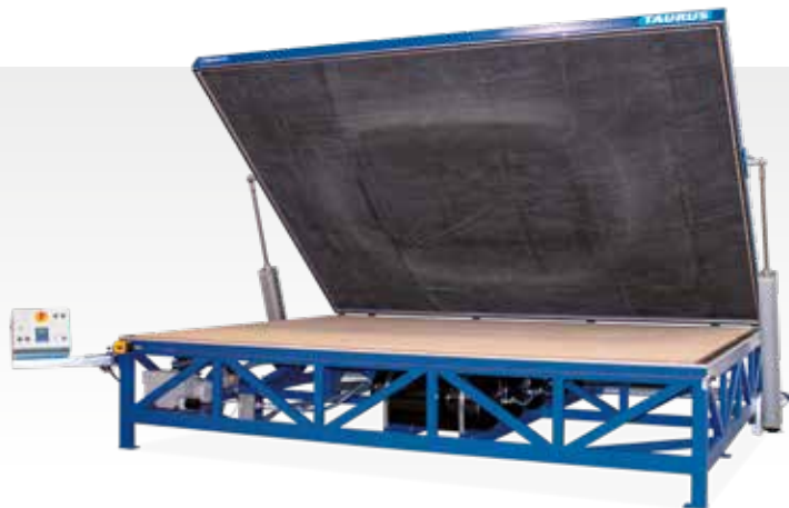
Upon request with pneumatic or hydraulic membrane opening
