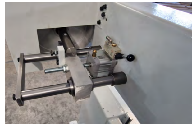
PNEUMATIC BELT TENSIONER (optional) Our large pneumatic belt tensioner guarantees excellent tension for all types of belts, with simplicity and speed of belt change.
